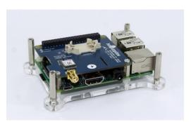
Finally attached the top pespex case with the supplied metal screws:
