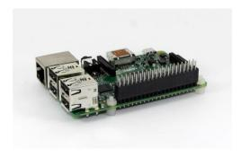
Place the expansion board on top of the header and push into place (it seats with a click). Screw two of the metal screws supplied with the expansion board into the metal hex spacers.
